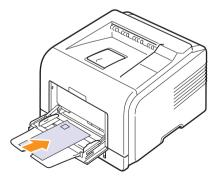
Squeeze the multi-purpose tray paper width guides and adjust them to the width of the paper. Do not force too much, or the paper will be bent, which will result in a paper iam or skew.
